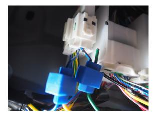
9) Connect cables using the scotch locks (or solder) please ensure the cables get a good connection
