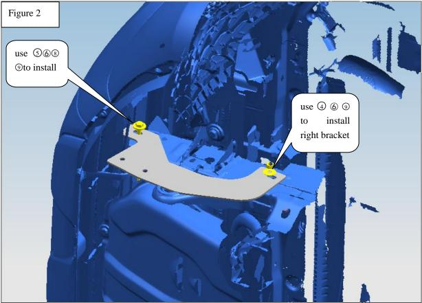
3. Connect the brackets and bar with thread according to following instruction, here you will see the bar will interfere the plastic plate underneath the vehicle. Line up the bar towards the plastic plate, mark the interferential area on the plastic plate,
